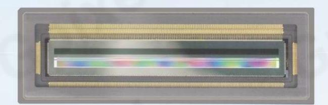
**GLT5009BSI** is a Backside illuminated (BSI), Time delay integration (TDI), charge domain CMOS image sensor with 5 μm pixels and 9k resolutions. The sensor has two photosensitive bands, 256 stages and 32 stages respectively, enabling a high dynamic range (HDR) imaging mode.
