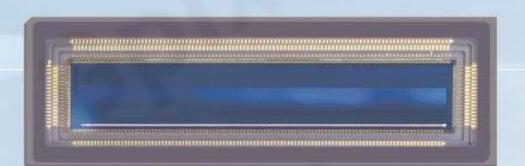
Designed for high speed industrial inspection, GL0816 is a line scan CMOS image sensor which consists of 16 lines of 8322 pixels with 5 µm pixel size and 5 µm inter-line space. It supports dual line, 4-line readout and max 8-line with 2-stage on-chip TDI.
