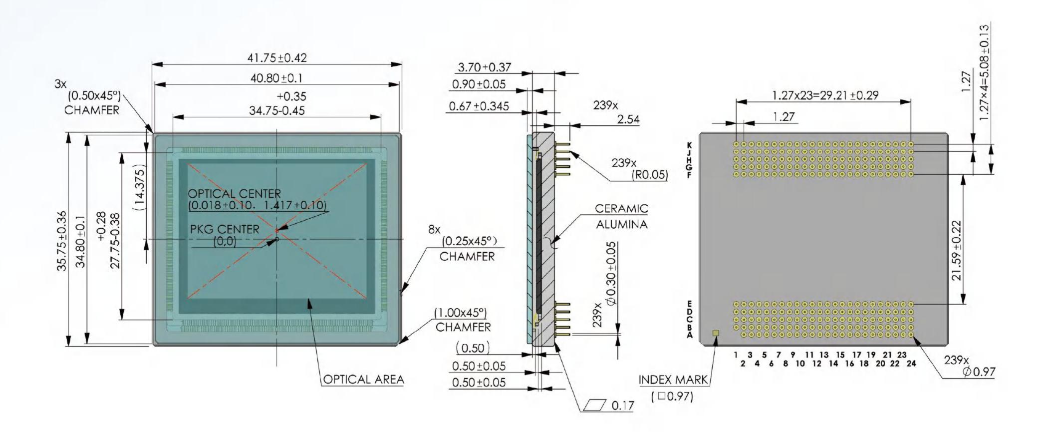
**GMAX32103** is a 103 Megapixel (11276 x 9200) medium-sized (46.6 mm) ultra-high resolution, global shutter image sensor designed with the latest 3.2 μm charge domain global shutter pixel. It achieves more than 9k e<sup>-</sup> FWC at low gain and 2.8 e<sup>-</sup> read noise at high gain separately with 66.4 dB intra-scene dynamic range. Using advanced 65 nm CIS process and light pipe technology, sensor achieves 66.9% peak QE (500 nm) and more than 1/15,000 shutter efficiency.
