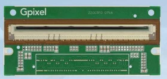
**GL7008** is a global shutter line scan image sensor with 7 µm square pixel and 8192 horizontal pixels resolutions. The sensor's 12 bit ADC transmits data over 25 pairs of Sub-LVDS at line rate up to 200 kHz. GL7008 is offered in both color and monochrome versions. The monochrome sensor supports single/dual/triple/quad line modes with optimal sensitivity.
