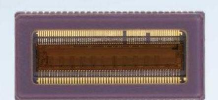
**GL3504** is a line scan image sensor suitable for small format camera integration with C mount lens, the sensor contains two lines with 3.5 μm pixel and four lines with 7 μm pixel. GL3504 could run up to 172 kHz with 7 μm pixel line and 84 kHz with 3.5 μm pixel line at 12 bit output with single line readout.
