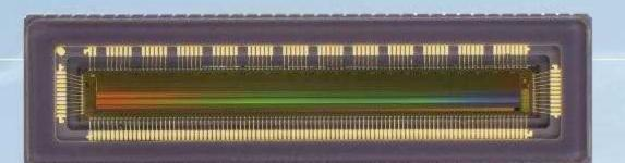
**GL0402** is a 4096 x 2 resolution, 7 μm square pixel, global shutter linear image sensor that supports maximum 200 kHz line rate in single line mode and 100 kHz line rate in dual line mode. GL0402 offers low read noise of less than 5.2 e<sup>-</sup> and 10 ke<sup>-</sup> FWC, leads to 65.6 dB intra-scene dynamic range.
