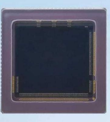
GLUX9701BSI a 1" sized, high sensitivity BSI sCMOS image sensor with a resolution of 1.3 MP (1280 x 1024) and large 9.76 μm x 9.76 μm pixels. Sensor supports a dual-gain HDR mode, achieving dynamic range of 89.5 dB by combining 1.6 e<sup>-</sup> readout noise. A dedicated low noise mode further optimizes imaging performance with read noise of 0.85 e<sup>-</sup> and power consumption of only 122 mW.
