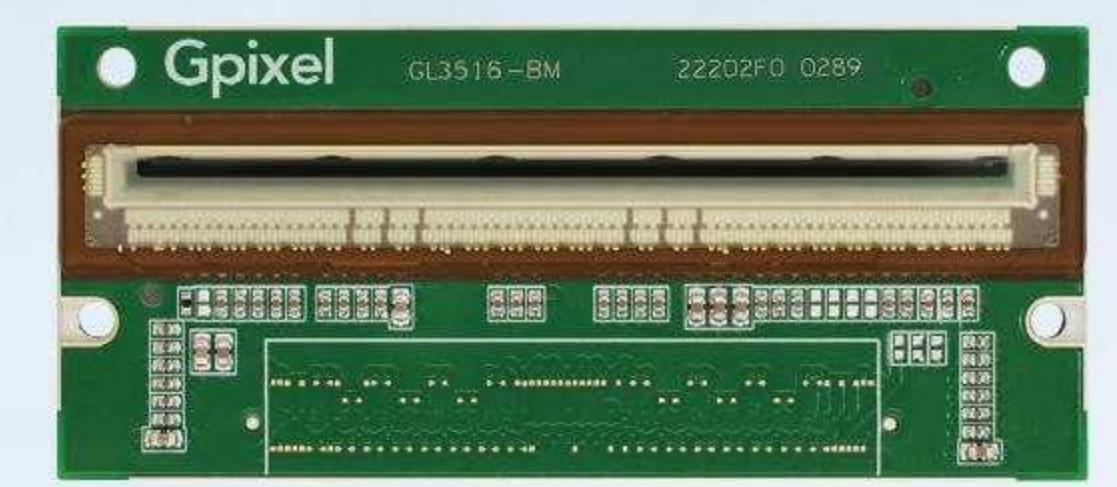
**GL3516** is a 16384 x 2 resolution, 3.5  $\mu\text{m}$  square pixel, line scan CMOS image sensor that supports maximum 120 kHz line rate in single line mode and 60 kHz line rate in dual line mode.
