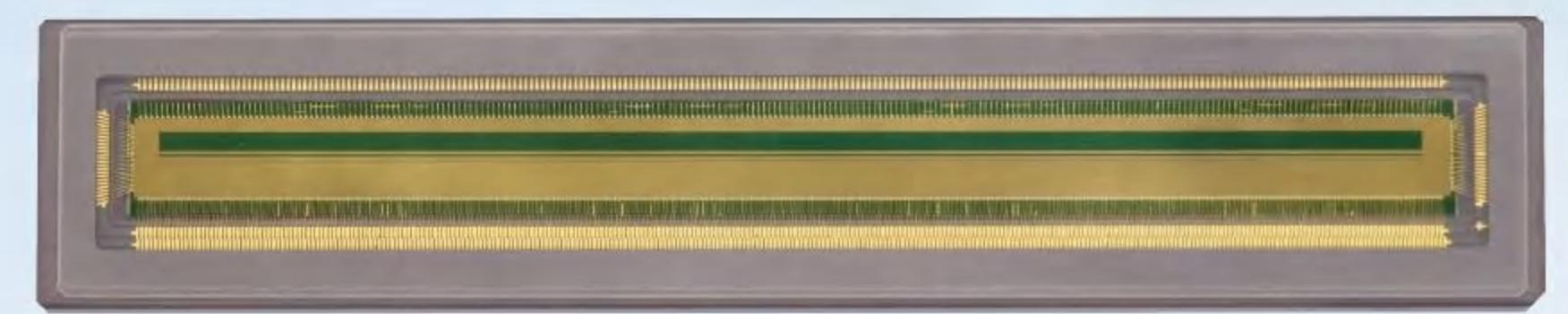
**GLT5016BSI** is a Backside illuminated (BSI), Time delay integration (TDI), charge domain CMOS image sensor with 5  $\mu\text{m}$  pixels and 16416 effective resolutions. The sensor has two photosensitive bands, 256 stages and 32 stages respectively enabling a high dynamic range (HDR) imaging mode, which is designed to meet the needs of high speed and low light applications by maximizing sensitivity with state-of-art BSI scientific CMOS technology.
