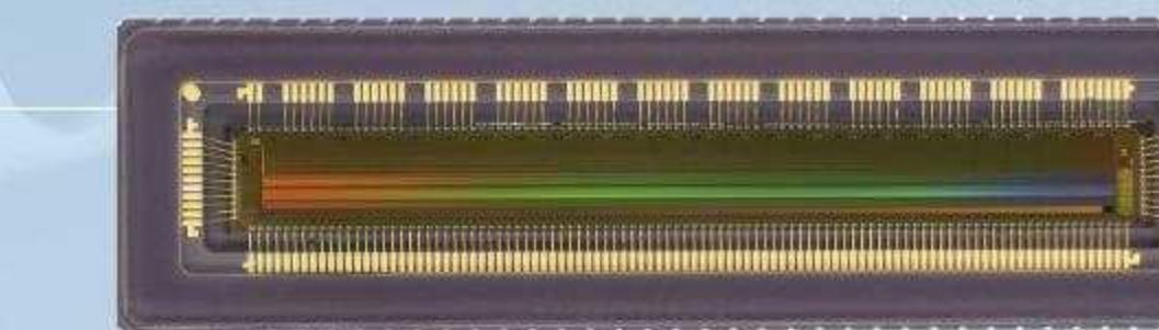
**GL0402** is a 4096 x 2 resolution, 7  $\mu\text{m}$  square pixel, global shutter linear image sensor that supports maximum 200 kHz line rate in single line mode and 100 kHz line rate in dual line mode. GL0402 offers low read noise of less than 5.2 e<sup>-</sup> and 10 ke<sup>-</sup> FWC, leads to 65.6 dB intra-scene dynamic range.
