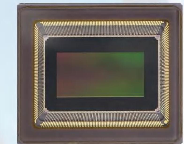
Featured with world smallest charge domain global shutter pixel, GMAX2509 is the new member of GMAX series C-mount line up after GMAX0505. It offers 4K (4200 x 2160) resolution in 2/3" optical format, operates with true CDS for low noise and high dynamic range. In addition, it has excellent PLS and angular response thanks to the light pipe technology.
