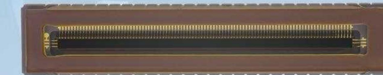
**GL1402** is available in color and mono variants. GL1402 color features red, green, and blue rows with 14  $\mu\text{m}$  gaps between each row to minimize color crosstalk. Readout speed is 27 kHz. GL1402 mono features a three row monochrome option with a readout speed of 27 kHz, or a one row monochrome option with a readout speed of 81 kHz.
