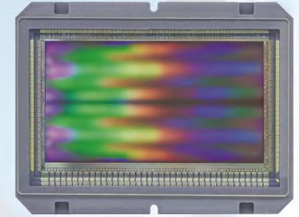
**GMAX32152** is an ultra-high resolution global shutter CMOS image sensor in medium format. Using a state-of-the-art charge domain pixel architecture, this sensor delivers an attractive combination of high frame rate and high dynamic range. A native 12 bit performance pixel achieves 67.3 dB dynamic range, combined with a high speed sub-LVDS delivering 16 fps. Pixel data is read out over serial differential pairs, with source synchronous clock and control channel.
