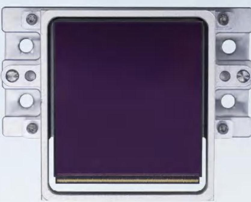
**GSENSE1081BSI** is designed with large imaging area for demanding scientific imaging applications. Sensor provides active resolution of 8900(H) x 9120(V) with 10  $\mu$ m x 10  $\mu$ m pixel size. An inter-scene dynamic range is 84.5 dB combined from maximum full well capacity of 90.68 ke<sup>-</sup> and readout noise of 5.35 e<sup>-</sup>.
