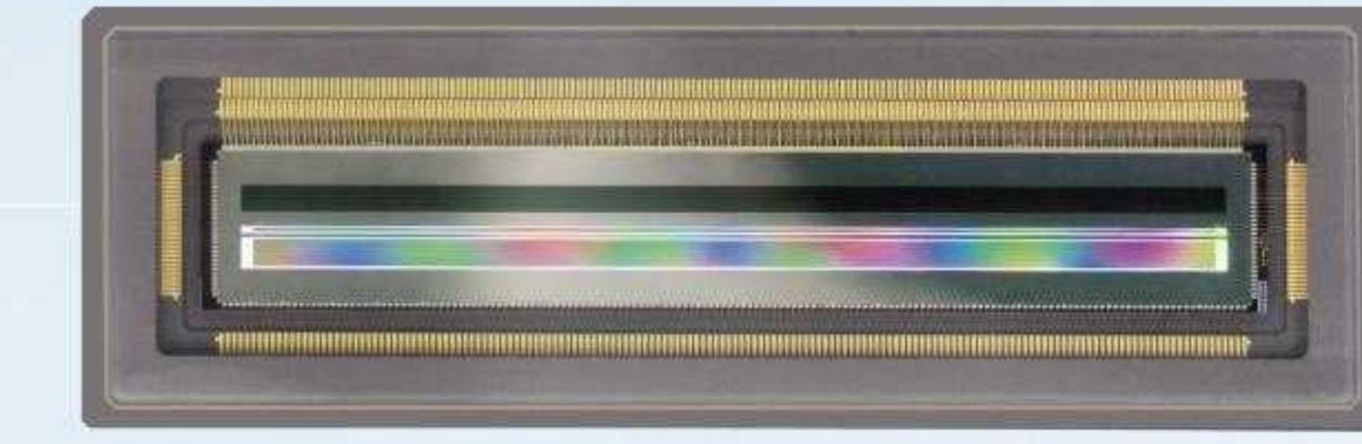
**GLT5009BSI** is a Backside illuminated (BSI), Time delay integration (TDI), charge domain CMOS image sensor with 5  $\mu\text{m}$  pixels and 9k resolutions. The sensor has two photosensitive bands, 256 stages and 32 stages respectively, enabling a high dynamic range (HDR) imaging mode.
