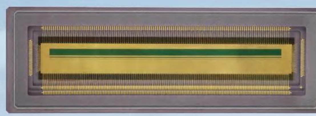
**GLT5008BSI** is a Backside illuminated (BSI), Time delay integration (TDI), charge domain CMOS image sensor with 5  $\mu$ m pixels and 8208 effective resolutions. The sensor has two photosensitive bands, 256 stages and 32 stages respectively enabling a high dynamic range (HDR) imaging mode, which is designed to meet the needs of high speed and low light applications by maximizing sensitivity with state-of-art BSI scientific CMOS technology.
