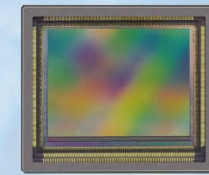
Featured with the latest generation 3.2  $\mu\text{m}$  charge-domain global shutter pixel and 65 MP (9344 x 7000) resolution, GMAX3265 is the leading-edge image sensor with 37.4 mm diagonal for high resolution machine vision and industrial inspection applications. This new generation pixel operates with true correlated double sampling (CDS), allowing low read noise and high dynamic range. In addition, the dual light pipe technology provides excellent PLS and angular response.
