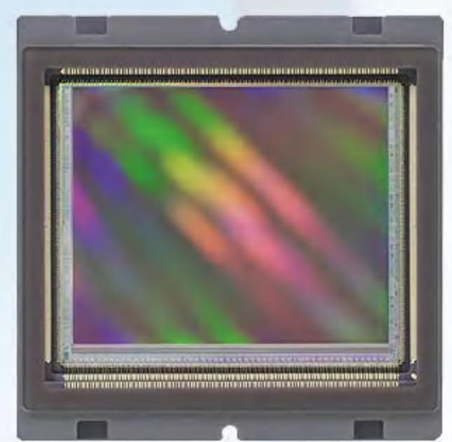
**GMAX32103** is a 103 Megapixel (11276 x 9200) medium-sized (46.6 mm) ultra-high resolution, global shutter image sensor designed with the latest 3.2  $\mu\text{m}$  charge domain global shutter pixel. It achieves more than 9k e $^-$  FWC at low gain and 2.8 e $^-$  read noise at high gain separately with 66.4 dB intra-scene dynamic range. Using advanced 65 nm CIS process and light pipe technology, sensor achieves 66.9% peak QE (500 nm) and more than 1/15,000 shutter efficiency.
