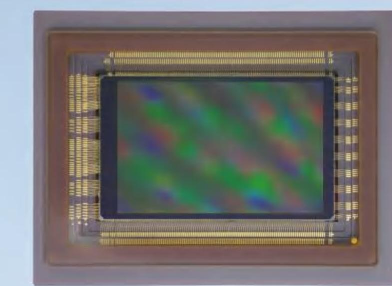
**GCINE3243** is a 43 MP  $26.2 \times 16.7$  mm<sup>2</sup> sized APS-style image sensor with a  $3.2 \mu\text{m}^2$  BSI pixel size designed specifically for the demands of high-end video imaging. With a resolution of 8192 x 5232 pixels and highly configurable read out, 8K video at 60 fps or binned 4K video at 120 fps is supported, all at an impressive bit depth of up to 14 bits per pixel. Readout of the image data occurs over 32 Sub LVDS channels (1.05 Gbps/channel).
