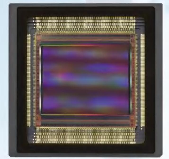
**GSPRINT4521** is a 21 MP (5120 x 4096) APS sized (29.5 mm diameter) high speed, global shutter image sensor designed with the latest 4.5  $\mu\text{m}$  charge domain global shutter pixel. It achieves 32  $\text{ke}^-$ , less than 3  $\text{e}^-$  rms read noise and >69 dB dynamic range, optionally increased to 81 dB with a dual gain HDR mode. Its state-of-the-art 65 nm CIS process allows the sensor to use on-chip charge binning, further increasing FWC and almost quadrupling frame rate.
