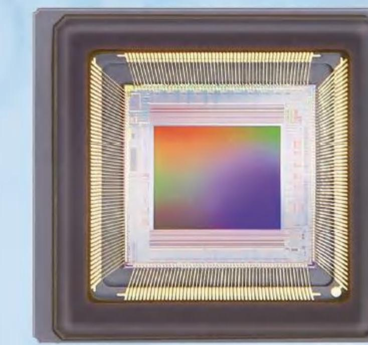
Featured with world smallest charge domain global shutter pixel, GMAX2505 is the new member of GMAX series C-mount line up after GMAX0505. It offers 5 MP (2600 x 2160) resolution in 1/2" optical format, operates with true CDS for low noise and high dynamic range. In addition, it has excellent PLS and angular response thanks to the light pipe technology.
