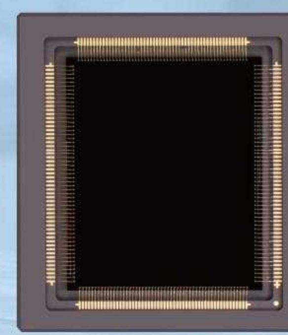
**GSENSE2020BSI** is a backside illuminated (BSI) scientific CMOS image sensor, with 4 MP resolution and 6.5  $\mu\text{m}$  pixel size. With six-transistor (6T) pixel architecture, GSENSE2020BSI features readout noise of  $1.6 \text{ e}^-$ , full well of  $55 \text{ ke}^-$ , as well as peak QE of 95%. In addition, the sensor supports correlated multiple sampling (CMS), the read noise can be further reduced to  $1.2 \text{ e}^-$  with 2-CMS operation.
