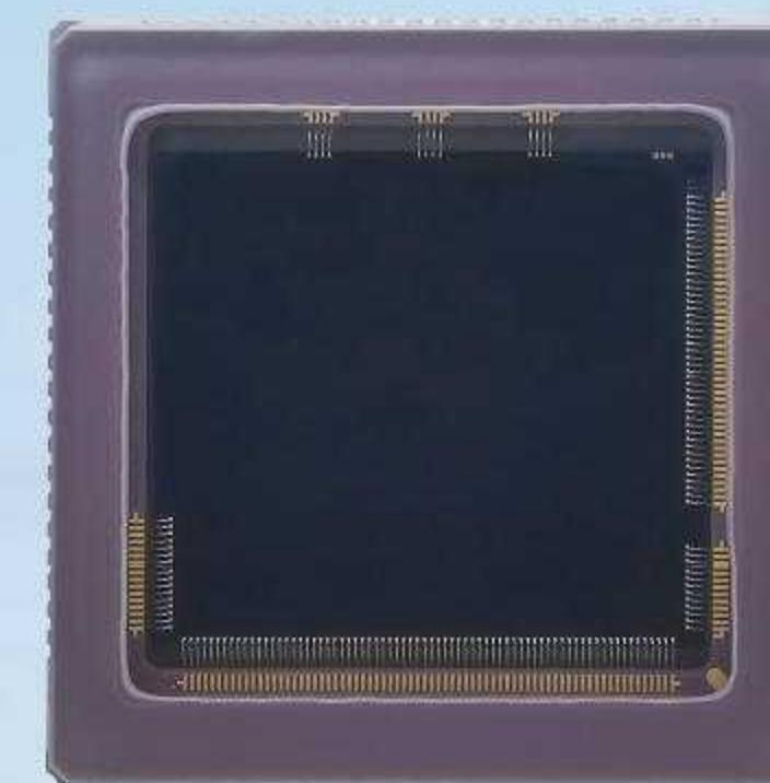
**GLUX9701BSI** a 1" sized, high sensitivity BSI sCMOS image sensor with a resolution of 1.3 MP (1280 x 1024) and large 9.76  $\mu\text{m}$  x 9.76  $\mu\text{m}$  pixels. Sensor supports a dual-gain HDR mode, achieving dynamic range of 89.5 dB by combining 1.6  $\text{e}^-$  readout noise. A dedicated low noise mode further optimizes imaging performance with read noise of 0.85  $\text{e}^-$  and power consumption of only 122 mW.
