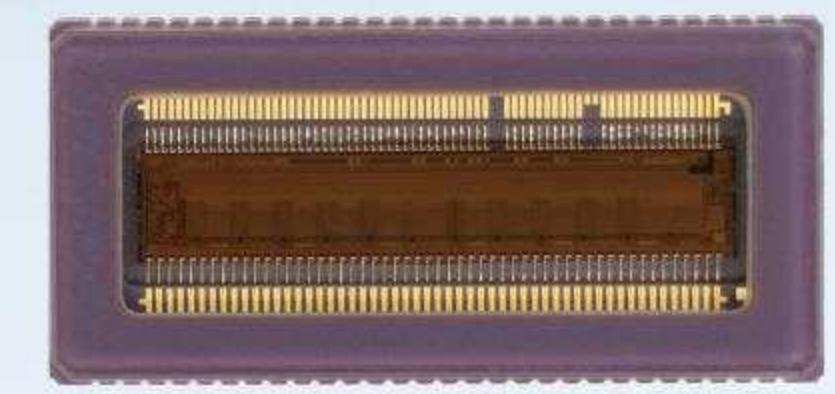
**GL3504** is a line scan image sensor suitable for small format camera integration with C mount lens, the sensor contains two lines with 3.5  $\mu\text{m}$  pixel and four lines with 7  $\mu\text{m}$  pixel. GL3504 could run up to 172 kHz with 7  $\mu\text{m}$  pixel line and 84 kHz with 3.5  $\mu\text{m}$  pixel line at 12 bit output with single line readout.
