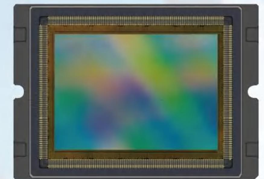
**GMAX4651** is a 51 Megapixel (8424 x 6032) full frame (35 mm) global shutter image sensor designed using the latest 4.6  $\mu\text{m}$  charge domain global shutter pixel. Using the advanced 65 nm CIS process, it provides 18 ke $^-$  FWC, 7.6 e $^-$  median dark noise and more than 65.5 dB intra-scene dynamic range. With the light pipe technology, sensor achieves > 67% QE (510 nm) and 1/40,000 shutter efficiency.
